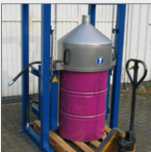
Beheizte Reststoffverdampfung aus 200 l Fässern Heated vaporization of waste material for 200 l drums
